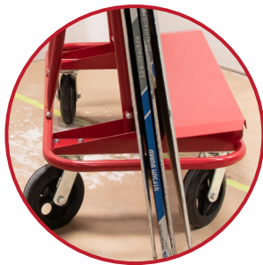
Sloped bed transports boards efficiently
