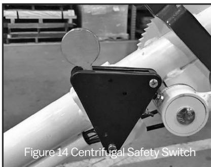
Figure 14 Centrifugal Safety Switch
