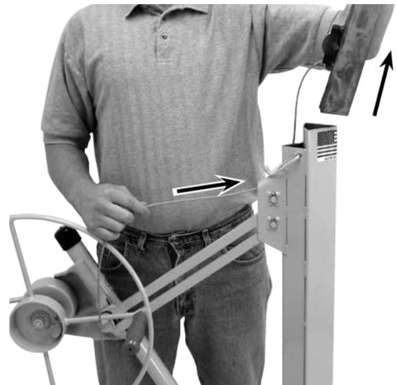
3. Remove the two telescoping sections completely from the frame housing. Pull the cable completely out from the frame along with them. Remove the "A" Section from the "B" Section as shown below. BE CAREFUL for loose strands or frays on the cable.
