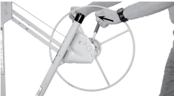
**3.** To lower the MARSHALLTOWN Drywall Lift control the backward rotation of the winch by grasping the winch handle with your right hand BEFORE releasing the brake with your left hand. ALWAYS use this two hand method when lowering the MARSHALLTOWN Drywall Lift.
