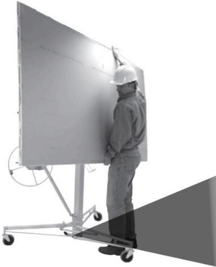
When the backstop legs are set, they keep the unit from shifting while loading wallboard or while installing the frame on the tripod base.
