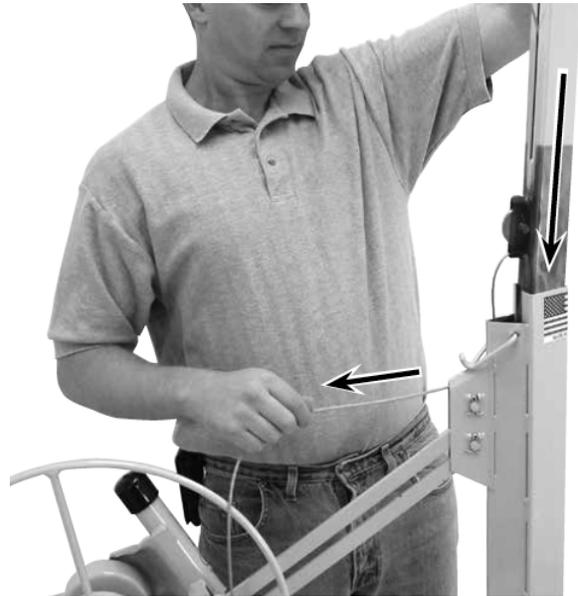
6. Pull the slack cable through the sheave pocket and slide the telescoping sections into the frame housing.
