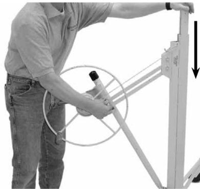
6. While holding the slide bar lock in this disengaged position with your right hand, push down on top of the telescoping section with your left hand. This action will cause the winch assembly to move toward the frame.
