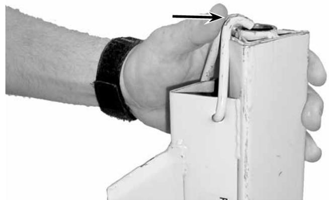
7. With the telescoping section all the way down, position the retaining hook over the top as shown.
