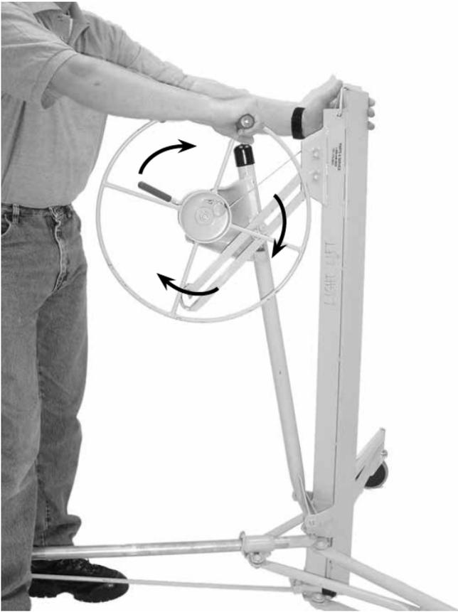
**8.** Hold the retaining hook in this position with your left hand and rotate the winch forward with your right hand. This will cause the winch assembly to fold up against the frame. When the slide bar contacts the frame, tighten the cable just sufficiently to hold the winch in the collapsed position.
