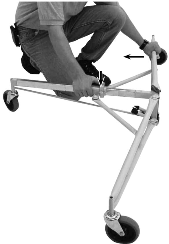
**10.** To collapse the tripod base, press down on the slide yoke pin clip and swing the legs in until they lock in the closed position.
