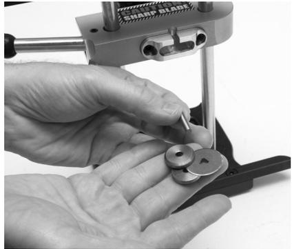
**Step 4** - Discard the old Blade and place a new one into the Axle Pin with a Spacer on either side of the Blade.
