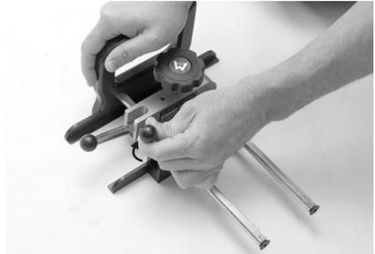
**Step 2** - Unlock guide fence (B) by lifting latch lever (C).
