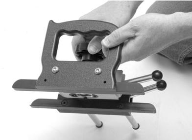
**Step 1** – Retract blade by turning depth knob (A) counterclockwise. You can stop when blade is fully retracted into the receiver. Continue to rotate knob if you would like to remove it completely.
