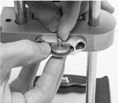
**Step 3** – Slide the Blade and Spacers out of the Blade Cartridge.
