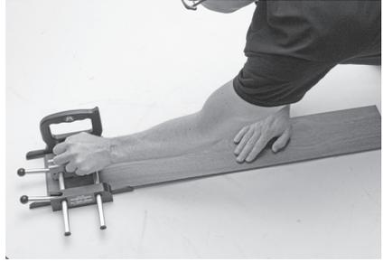
**Step 12** - Slide the Ripper off the end of the plank.
