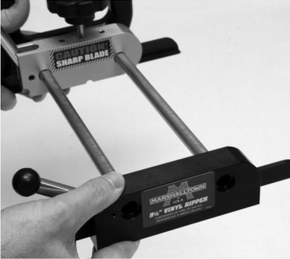
**Step 5** - Attach Guide Fence (C) to Guide Rods (D) with the Latch Lever facing the same direction as Blade Receiver's (B) Latch Lever.
