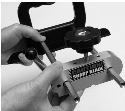
**Step 4** – Slide Blade Receiver (B) onto Guide Rods (D) so that the Latch Lever is facing you and Carry Handle (A) is on the left.
