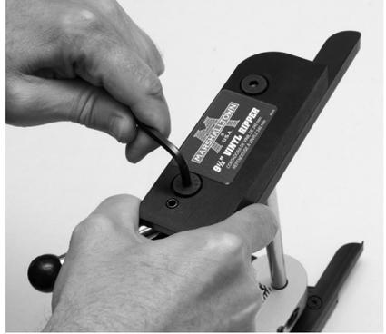
**Step 6** - Install and tighten Screws (F) into Guide Rods (D) using Hex Wrench (G).
