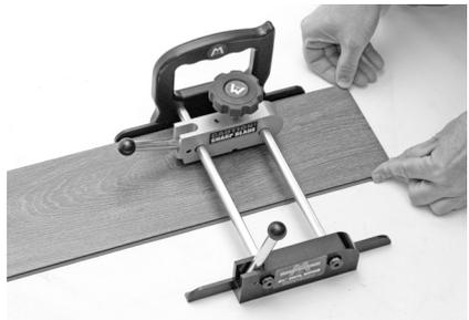
**Step 4** - Place the MARSHALLTOWN® Vinyl Ripper over a vinyl plank.
