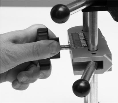
**Step 1** – Extend Blade Cartridge by turning the Handle Knob clockwise until it stops. Do not force the knob further.
