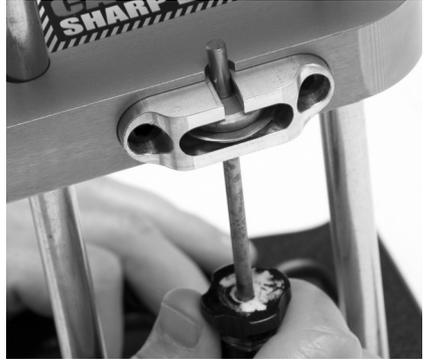
**Step 2** - Use a screwdriver or pen to push the Axle Pin out of the Blade Cartridge.
