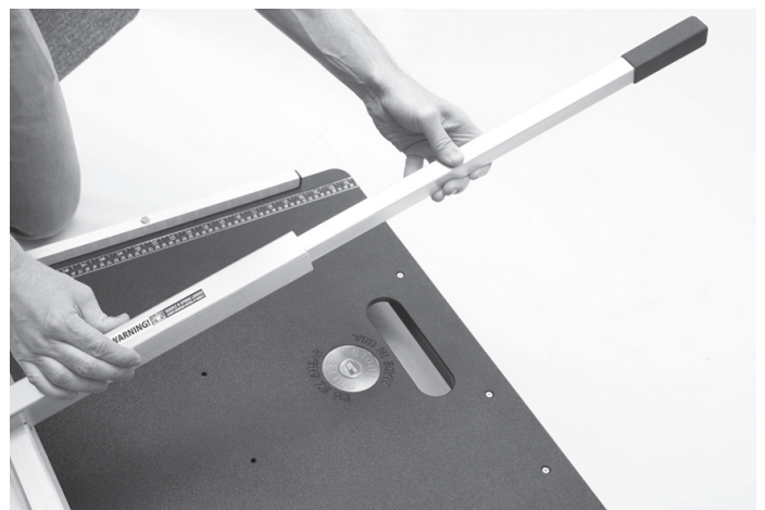
8. Attach the Handle (G) to the Handle Assembly (F).
