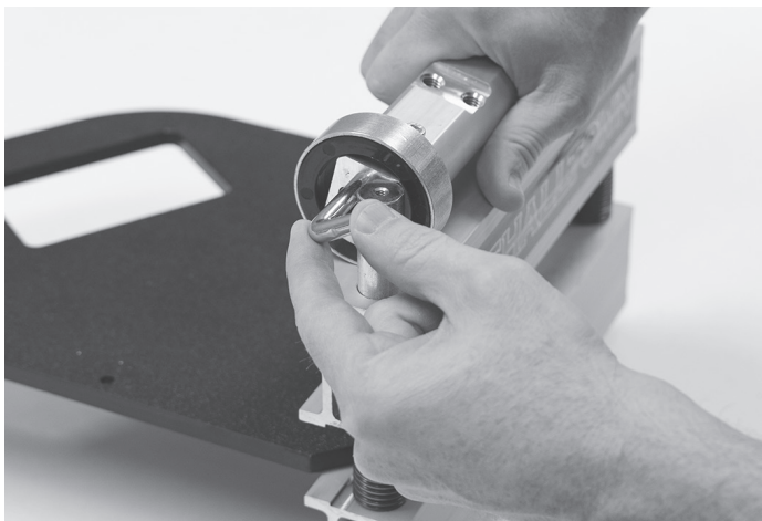
6. Rotate the Handle Base on the top of the Cutter Assembly (F) and insert the Locking Pin (G) into the side.
