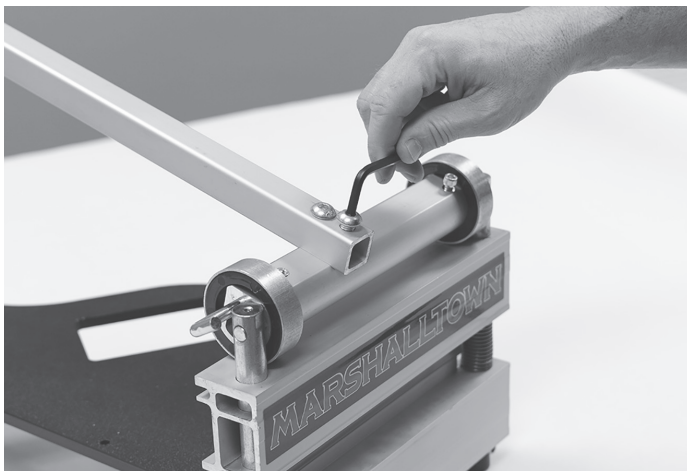
5. Attach the Bed (A) to the Cutter Assembly (F) using Hardware Set (I) for the back and Hardware Set (H) for the front.
