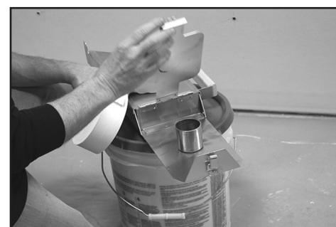
1. With mud compartment door facing up, lay Pro "Quick-Load" Drywall Taper on side.
