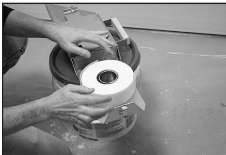
**5. Hand feed tape into rear slot of mud compartment, threading 8 to 12".**
