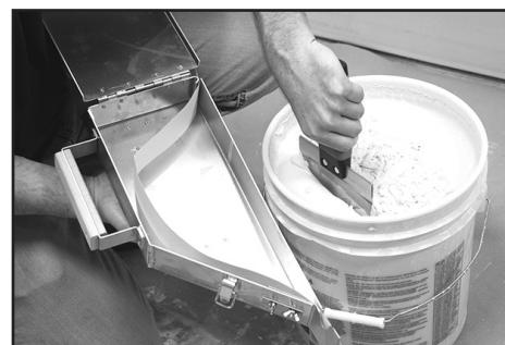
**9. In order for tape to skim across surface of mud, mold tape from bottom to top and along sides of mud compartment.**
