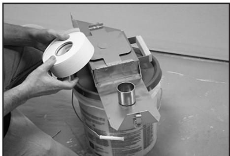
**4. Place roll of tape on tape spool, unreeling in clockwise direction.**
